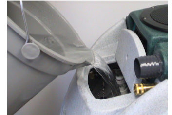
Pour 2 or 3 gallons of clean water into Solution Tank
